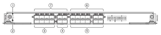
Figure 24. FX8-24 extension blade
